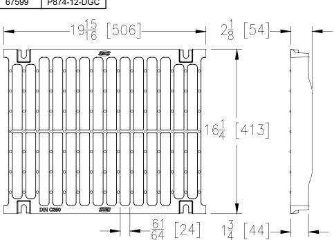
**DGC GRATE ENGINEERING SPECIFICATION:** The Zurn P874-12-DGC Slotted Grate, Ductile Iron, is 16-1/4" [413mm] wide by 19-15/16" [506mm] long, weighing 28 lbs per linear foot[41.4 kg/m]. The grate has an open area of 118 square inches per linear foot[2497 cm2/m], DIN Rating of C, ANSI Rating of Heavy-Duty, H-20 Load Rated. Ductile Iron Conforms to ASTM Specification A536, Grade 80-55-06.
